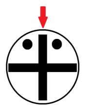
To the left is a depiction of the adjustment knob of POT1. You will see two dots on either side of the top of the plus sign (Phillips screwdriver slot), this is where the adjustment is currently set. Also indicated by the red arrow in the diagram. Simply use a precision or fine bit screwdriver to gently turn the adjustment knob to the desired setting. The charge current is adjustable from 0.7A – 1.5A. **Do not use electric screwdriver or drill.**
